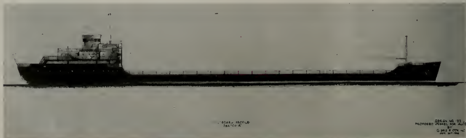
Climaxing years of intensive Alcoa research, the 10,000 ton all-aluminum ship shown above represents a new era in marine construction. Hull, superstructure, lifeboats and fittings will be fabricated from aluminum alloys pretested for resistance to salt water corrosion. Overall length of the carrier is 422 feet, extreme beam 60 feet.
